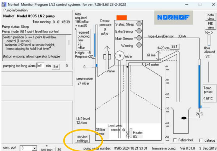
In service settings select the tab <calibration> click on the [calibrate 0 mBar] button
