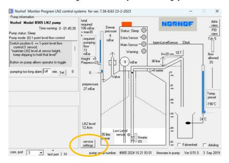
In service settings select the tab <calibration> click on both sensors the [calibrate -196] button
