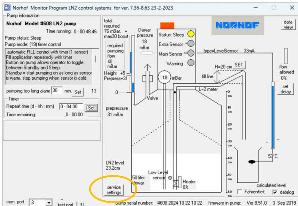
In service settings select the tab <calibration> click on the [calibrate -196] button
