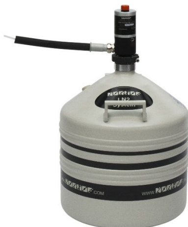
Norhof #608 pump, mounted on a 35 Liter Dewar
