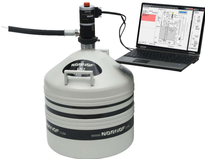
Norhof 900 series pump, mounted on a 35 Liter Dewar
